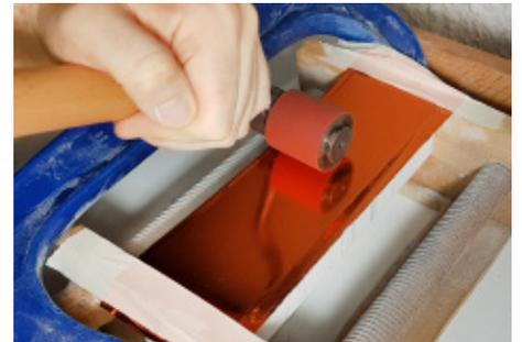
foil is carefully applied using a specialist heated roller and manual pressure...
