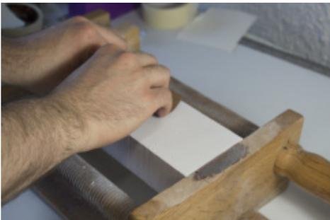
cards are clamped and carefully sanded until the entire stack is completely smooth...
